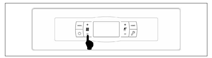
To select the circuit flow temperature, press **MENU** to browse until the **\$\frac{1}{2}** icon appears on the display with the **SET** symbol flashing. The temperature can be changed by pressing the "+" and "—" Heating symbols.
