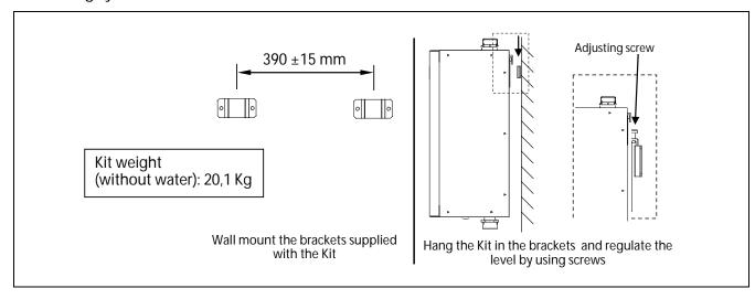
To assemble the Kit, with the flow and return boiler outlets on the bottom part, follow these steps:
