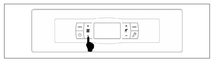
To select the circuit flow temperature, press **MENU** to browse until the **\$\frac{\pmathtarrow}{\pmathtarrow}\pmathtarrow}** icon appears on the display with the **SET** symbol flashing. The temperature can be changed by pressing the "\pm" and "\pm" Heating symbols.
